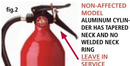
Those models that were manufactured with Zytel® (black plastic) valves and **aluminum** cylinders (see fig 2) are **not** affected and can remain in service.
